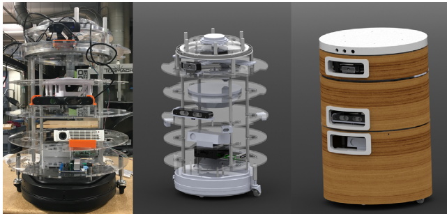
Figure 2: tbo's internal and external hardware design
