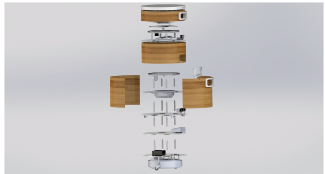
Figure 4: tbo is designed with easily accessible internals and empty "hackable" strata to add features
